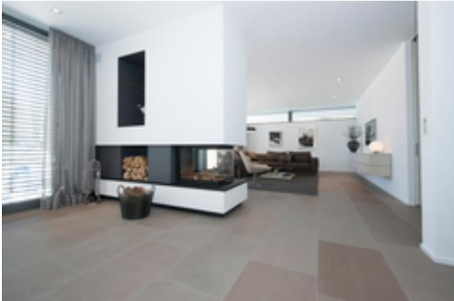
The Krefeld tiling professionals not only laid the 50 x 80 cm quartzite natural stone tiles throughout the ground floor, they also tiled the adjoining patio behind the floor-to-ceiling windows with tiles of the same size. The generous, continuous tiling concept supports the spacious, bright impression of the rooms, in particular in the living area.
